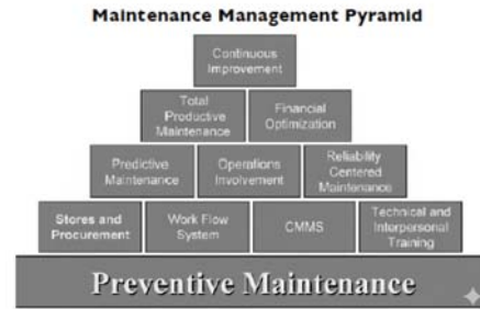
Figure 1. Maintenance Pyramid: Hierarchy of Maintenance Practices according to Wireman (2003). The structure demonstrates that advanced Reliability Engineering techniques at the top depend on well-established fundamental practices at the base.
