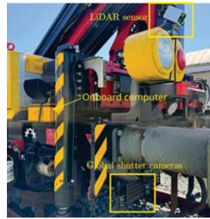
Fig. 2. AIRIS autonomous inspection hardware.
