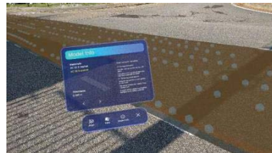
Fig. 6. AR-based visualization of GPR-derived pavement layer through HoloLens 2.
