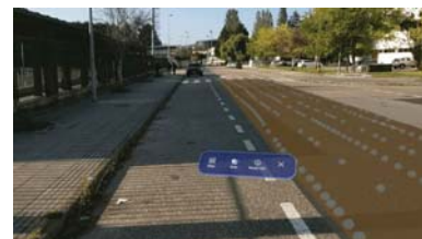
Fig. 7. AR-based visualization of GPR-derived pavement layers within the roadway context through HoloLens 2.
