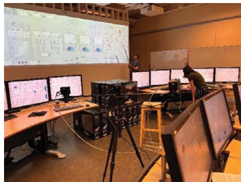
Fig. 1. Optitrack cameras setup for 3D modelling
