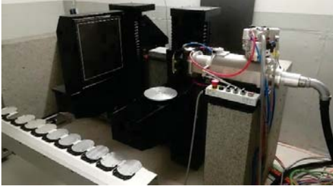
Fig. 2. Used \mu\text{-CT} system with transmission X-ray source and flat-panel detector (Source: diondo GmbH).
