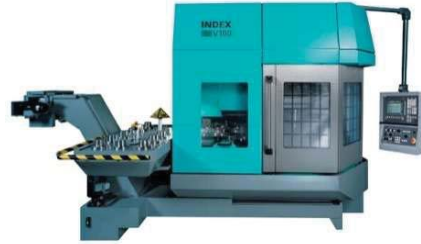
Figure 1. Full enclosure of an automatic vertical lathe in accordance with EN ISO 23125 (source: INDEX).
