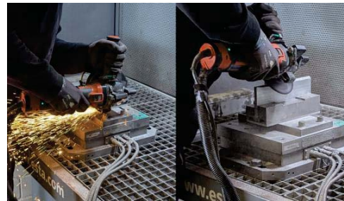
Fig. 7. Test run. Left roughing aluminium. Right cutting steel. Both material samples are the same size of 200 mm x 80 mm x 10 mm clamped and oriented in different ways.
