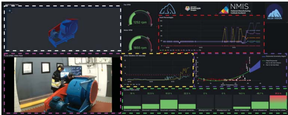
Fig. 6. HMI for unbalance scenario demonstration. White box – 3D model of fan skid; Pink box – Live video feed of the NMIS DPMC facility; Red box – Time-series of fault probability scores; Yellow box – Time-series of Fan 1X velocity vibration data; Purple box – Unbalance prognostic model; Green box – Histogram of probability percentages of diagnostic fault scenarios.
