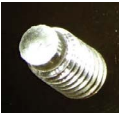
Fig. 6. Broken threaded pin (Napp 2026)
