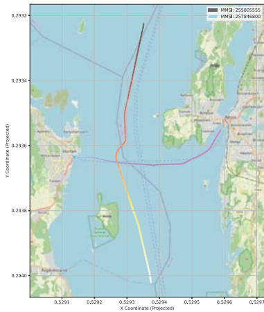
Fig. 7.: One of the identified crossing encounter situations where an outbound vessel from Oslo intersects with a ferry traveling from Horten to Moss. The outbound vessel performs an evasive maneuver to avoid collision. The trajectories are rendered in the Web Mercator projection (EPSG:3857), the standard projection used by OpenStreetMap.
