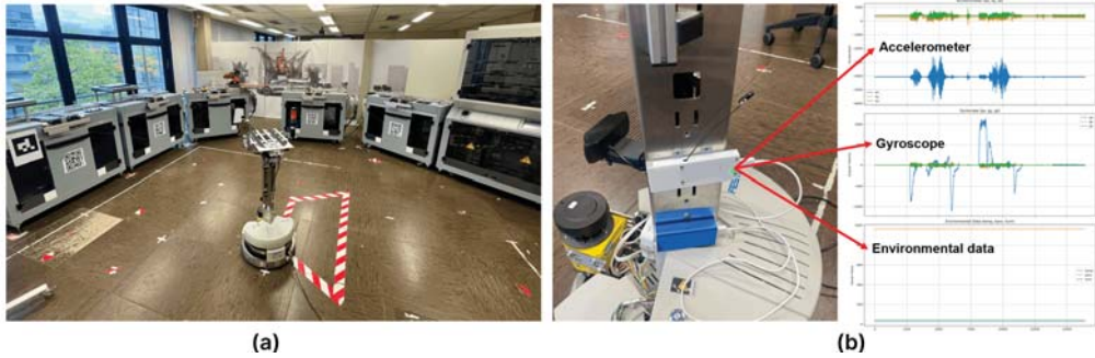
Fig. 2. Overview of the experimental setup and MEMS sensor with enclosure: (a) mobile robot operating in the test environment; (b) sensor mounting location on the robot and example accelerometer, gyroscope, and environmental sensor signals.
