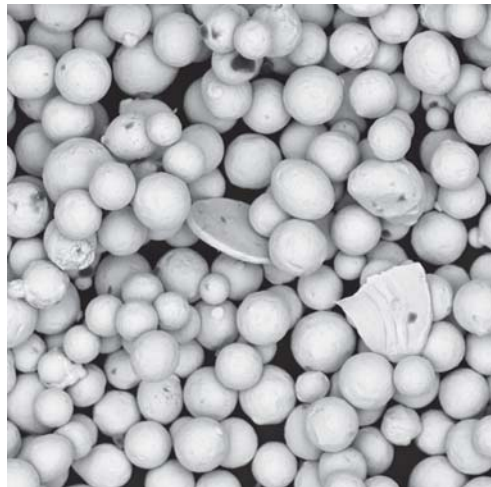
Fig. 2. Scanning electron microscope images of a purified solder paste: Deformed or destroyed solder balls
