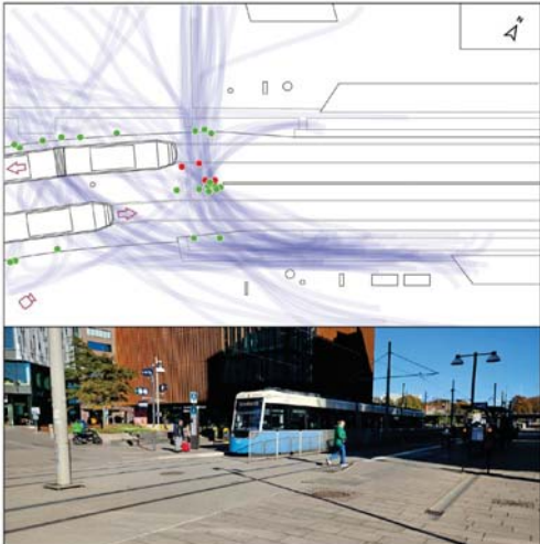
Fig. 6. Safety-critical situation at Gamlestadstorg caused by a stationary tram obstructing visibility.
