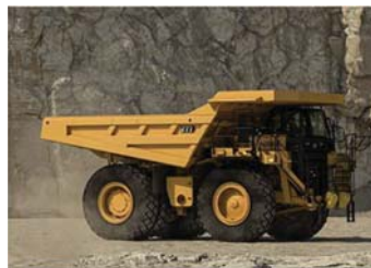
Figure 2. Cat Off-Highway Truck 777, by Caterpillar website.
