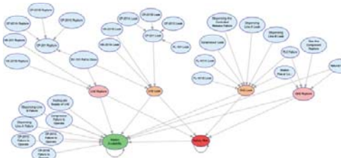
Fig. 3 LH2 Fueling Station DBN
