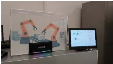
Fig. 4. Raspberry Pi-based digital twin prototype featuring a graphical user interface for interactive simulation of machine operational states, alarms, and maintenance events. An external audio speaker reproduces machine noise from pre-recorded audio signals acquired on real industrial machines.
