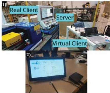
Fig. 3. 1) Data transmission layout; 2) Digital twin of machine on Raspberry Pi
