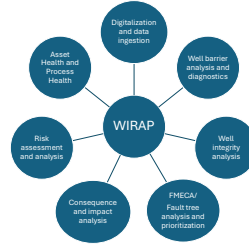
Fig. 1. Technical components of the integrated WIRAP platform.
