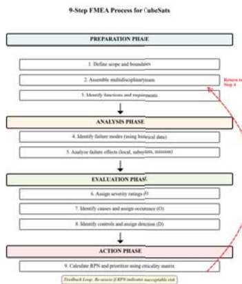
Fig. 2. Systematic 9-step FMEA process organized by phases, with iterative feedback loop for risk re-assessment.
