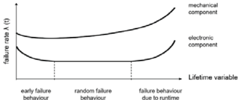
Fig. 1. Failure rate and characteristic failure behaviour for mechanical and electric components (bathtub curve).
