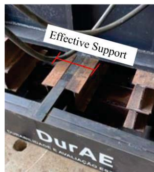
Fig.2. Steel box-type support device
